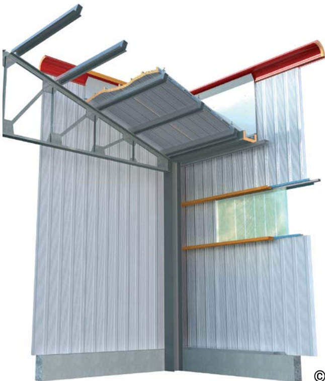
ROOF, WALL, GUTTER CONNECTION (bottom view)
