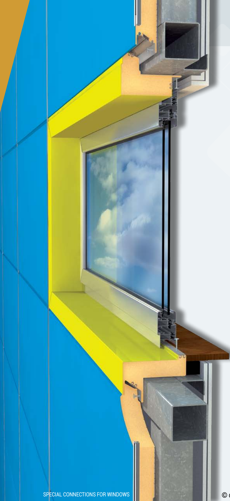
DETAIL TERMOPARETI® WALL JOINT
