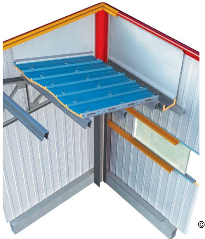
ROOF, WALL, GUTTER CONNECTION (top view)
